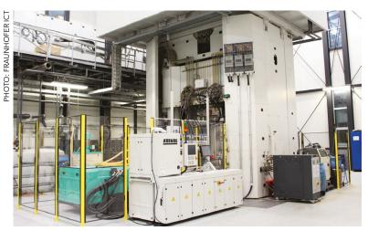
Above: A specially-designed Arburg injection unit with integrated Fibre Direct Compounding can be quickly connected to and disconnected from a Dieffenbacher vertical press
