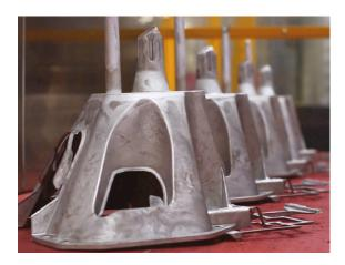
profiles show significantly higher dimensional stability as well as increased torsional strength and stiffness," says Lukas Schröer, Project Manager for lightweight structures in the company's High Performance Materials (HPM) business unit. "We believe that this new 'Hollow Profile Hybrid Technology' enables the manufacturing of components such as cross car beams, which up until now were not resilient enough using classic plastic-metal hybrid technology."
