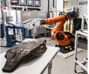
composites seat back was developed and produced during the MoPaHyb project
