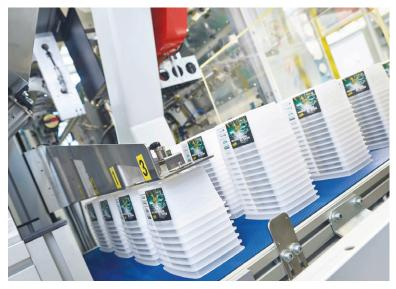
Above left: Arburg's hybrid Allrounder 820 H in the "Packaging" version debuted at Fakuma 2018. Above right: At the event, Arburg's hybrid Allrounder 820 H produced thin-walled IML containers in a four-cavity mould in a cycle time of around 3.8 s
